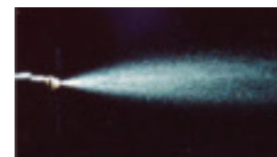
Injector spray pattern after P.i. treatment.
