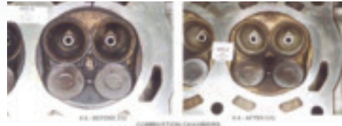
Combustion chamber before P.i. treatment. Combustion chamber after P.i. treatment.
