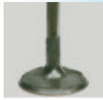
Intake valve after P.i. treatment.
